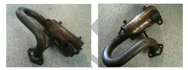
The muffler, header pipe and flange assembly cannot be altered in any way other than the outer surface finish (e.g. paint coating). Ceramic coating or any similar process will also render the muffler illegal.
